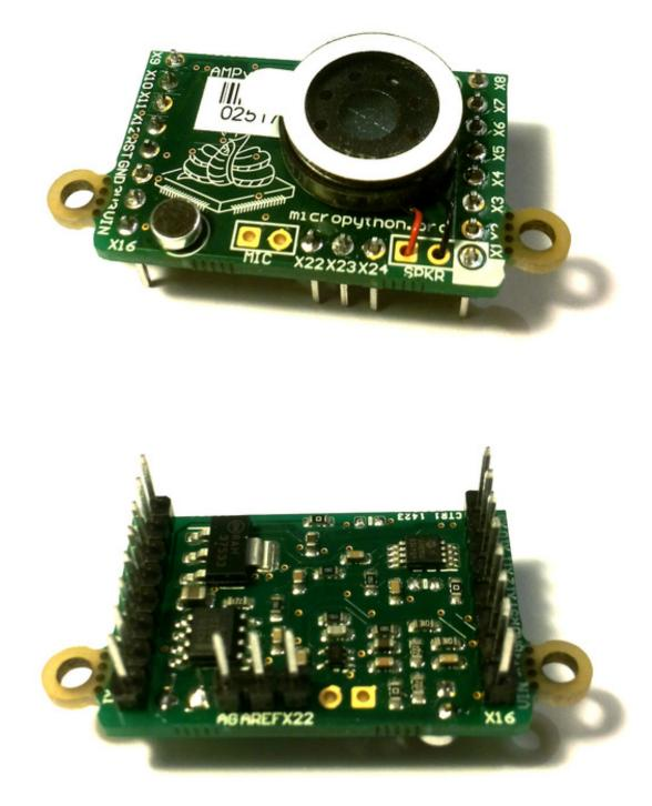
The following video shows how to solder the headers, microphone and speaker onto the AMP skin. For circuit schematics and datasheets for the components on the skin see *The pyboard hardware*.
