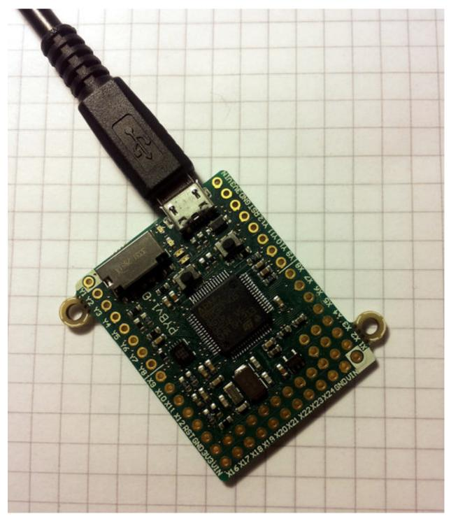
When the pyboard is connected to your PC it will power on and enter the start up process (the boot process). The green LED should light up for half a second or less, and when it turns off it means the boot process has completed.
