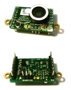
The following video shows how to solder the headers, microphone and speaker onto the AMP skin.
